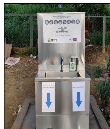
A foot pedal operated handwash station installed by Pragma
